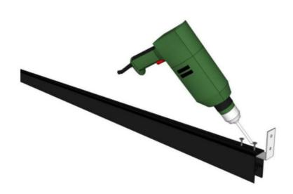
Before install steel holder, using the screws to make the combination between L bracket and Top rail (Bottom rail), like pictures.
