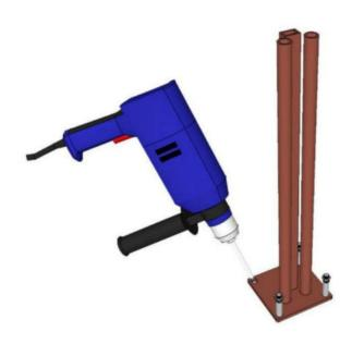
According to install request, Using the impact drill to make the holes on concrete ground and then put anchoring to fixing steel holder. Adjusting the distance between two aluminum posts.
