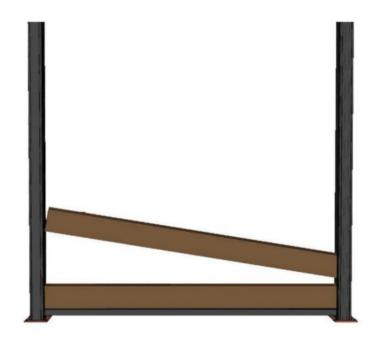
After install bottom rail, inserting the fence board directly, like picture.
