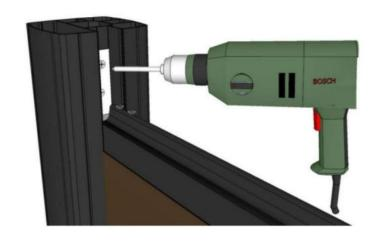
Using the impact drill to make holes then fixing top rail by screws.
